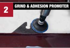
Grind repair on both sides at low RPM or by hand with P36 grit disc. Drill 1/8" holes in repair area to help "lock in" the repair material. Blow off surface.
