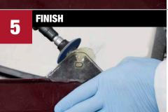
Grind the tab back to its original shape and size. Re-drill the bolt hole.
