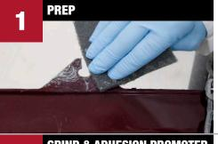
Clean front and back with Scuff & Clean and damp. gray scuff pad. Rinse with water and dry with clean, lint-free cloth. Clean front and back with SEM Solve, Plastic & Leather Prep or XXX Universal Surface Cleaner. Wipe clean in one direction with dry, lint-free cloth.
